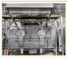
Further introduction of dyeing machines with a lower liquor ratio 進一步引進低浴比染缸
